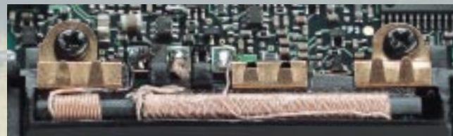
Internal ferrite bar antenna
